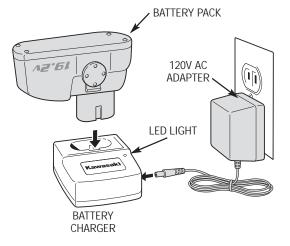
3. When fully charged, reattach battery pack onto Cordless Drill, making certain latches fasten securely. Cordless Drill will not operate properly if the battery pack is not seated properly.
